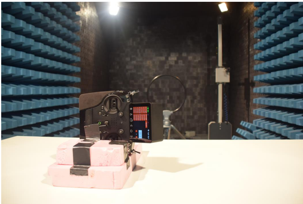
Picture 4: CDC, radiated emission test 9 kHz -30 MHz – position Z (front view)
