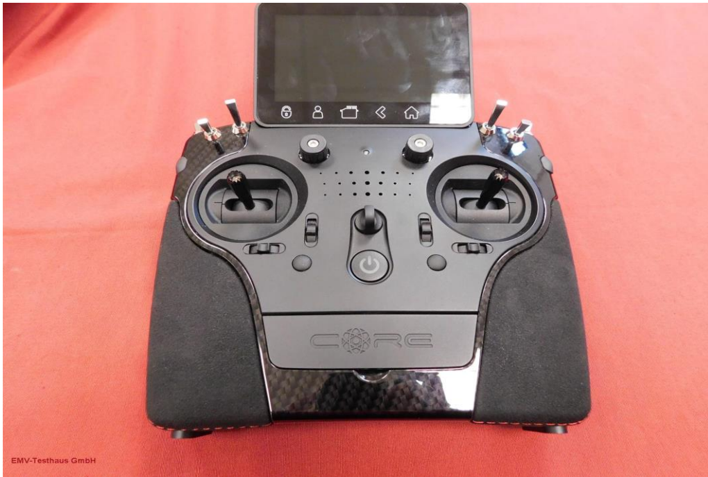
Picture 5: Top view of EUT for radiated measurements < 30 MHz
