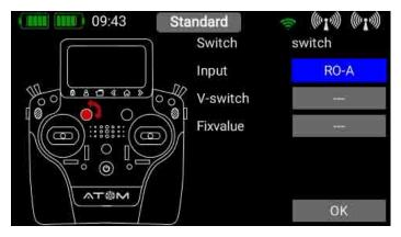
A further alternative is to define a fixed value - **On** or **Off**. This is necessary, for example, if you only wish to assign a switching threshold to one linear control. In this case select one transmitter control as fixed value, and define a linear control for the other transmitter control.
