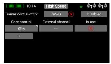
Repeat the procedure with the transmitter control from the Student transmitter: press the empty field under **External channel** and move the appropriate stick or switch at the Student transmitter. The Atom automatically detects which channel has been moved, and assigns this channel to the transmitter control at the **Atom**.
