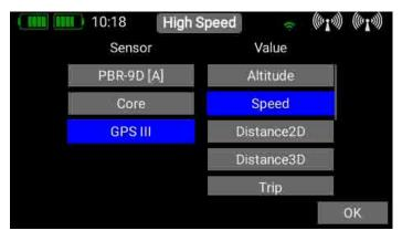
The left-hand column shows all the connected sensors, while the right-hand column shows all the values which these sensors supply. The **P2BUS** is an in-house development, and is capable of transmitting up to **255 sensors each with 32 individual values** – and at a speed of up to **800 values per second!**
