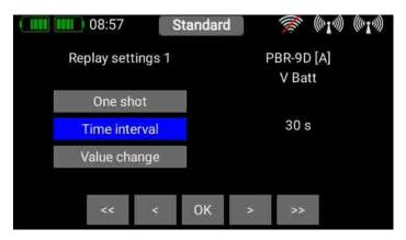
The **Once** option is used if you wish to have a timer or a telemetry value spoken when a switch is operated.
