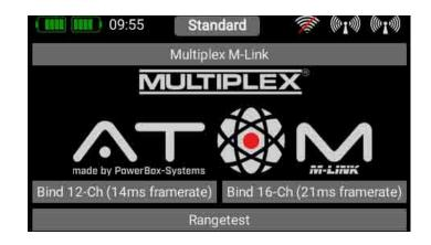
Choose your setting. If you do not need more than twelve channels, you should always give preference to **Option 12K**, as the servos are addressed at a higher rate in this mode. This can be advantageous in respect of smooth running, transit speed and precision. In contrast, **Option 16K** offers sixteen channels and a slower frame rate; this is the best choice for use with older servos.
