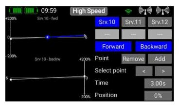
As you can see in the picture above right, an additional travel point has been added in the **Servo 10-Forward sequence**. You can now select the point you wish to alter using the arrow buttons after **Select point**.
