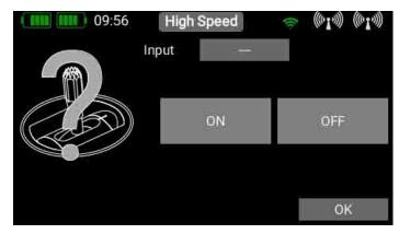
The transmitter control can be either a switch or a linear control. In both cases you can set the desired switching points and the switching direction. Please note that the green range covers the sequencer running **forward**, the red range the **reverse** range. More on this later when we discuss the method of setting travel points.
