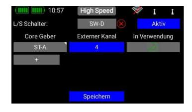
At top right there is a further button - **Active** or **Inactive**. This can be used to disable the Teacher / Student system completely, even if a Student receiver is still connected.
