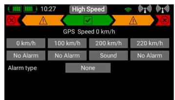
The final step is to select the type of warning you want. In our example a warning tone is set to be generated at 200 km/h, while a spoken message is generated at 220 km/h.
