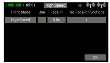
You can immediately assign an informative name to the new flight mode by briefly pressing the left-hand field. Bear in mind that you should not use abbreviations here if you intend the flight mode names to be used for speech output later, as the TTS systems reads the text exactly as you have entered it!
