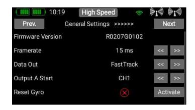
The **Next** and **Previous** buttons at top left and right can be used to navigate through any sub-menus which the sensor offers. Briefly pressing the **arrow** buttons to the right of the sensor values allows you to alter the sensor values. You can set larger values more quickly by keeping your finger on the **arrow** buttons. To leave the menu press the **∢**-button at the bottom of the touch-screen.
