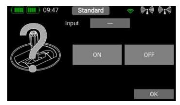
Yet another option is to use the output of a previously defined **logical switch** in turn as a transmitter control input. Press **OK** when you have made your selection. In the following section you will see your transmitter control on the left. Depending on whether you have selected a linear input or a switch, you will see one of these screens:
