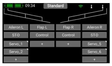
Briefly press Control, and move the aileron stick to select the Aileron control in the Context menu. Now you select a transmitter control which is to control the left aileron; this will be the left or right primary stick, depending on the transmitter mode you prefer.
