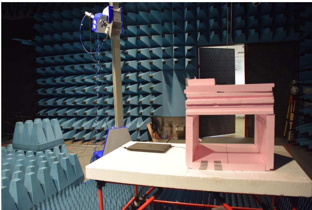
Picture 8: AC, radiated emission test 1 GHz – 17 GHz – position X (back view)
