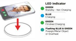
3. The charging pad's LED indicator will light up solid BLUE when your device is charging, and turn solid GREEN when your device is fully charged.
