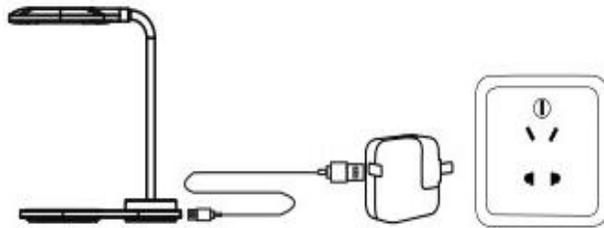
2. Put your phones onto the wireless charging area, phones starts to charge and indicator shows flashing blue color, once phones are full charged, blue indicator will keep lighting on.
