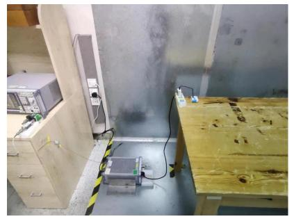
Radiated Spurious Emissions Test Frequency From 30MHz-1000MHz
