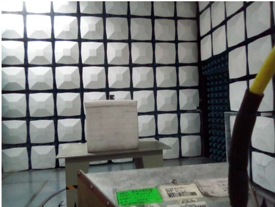
Radiated Emission View (Above 1GHz)
