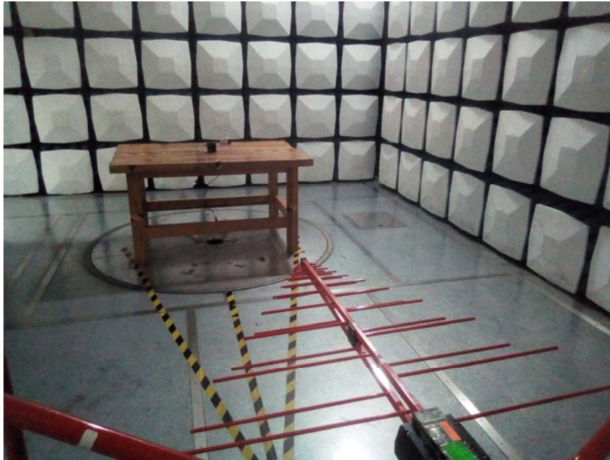
Radiated Emission View (Below 1GHz)
