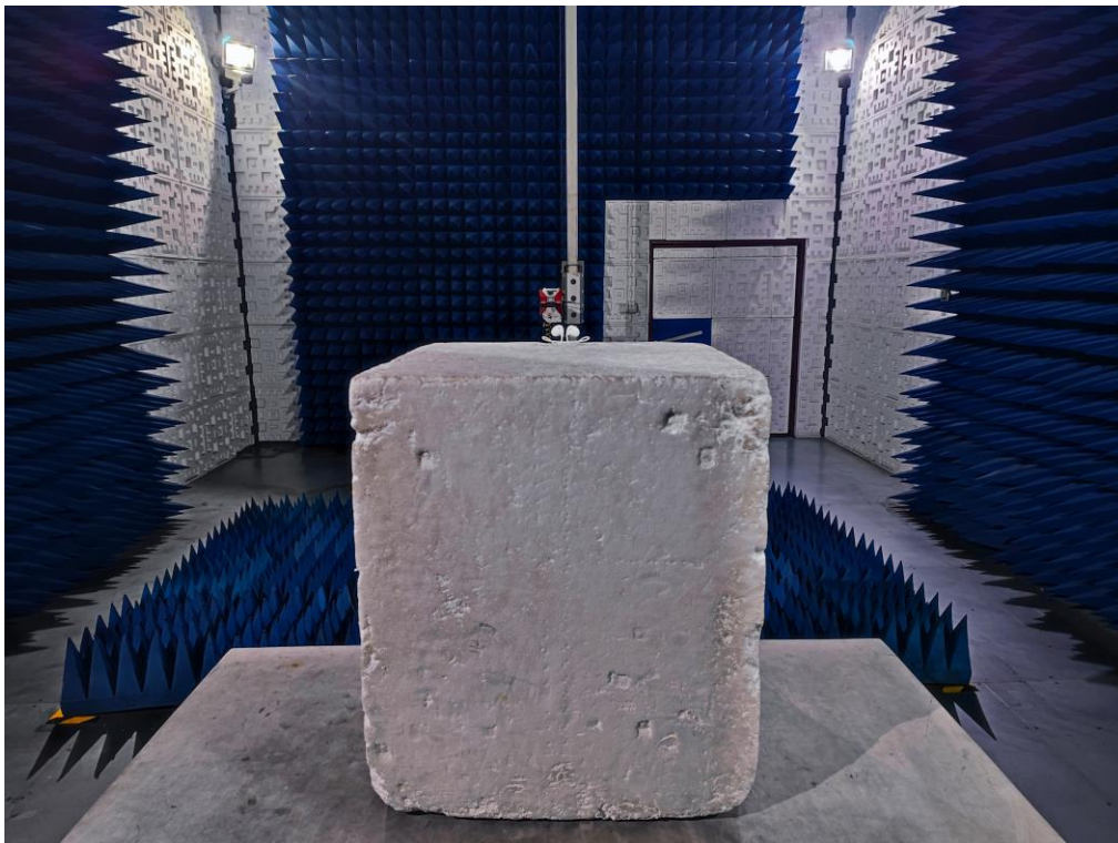
RADIATED EMISSION TEST SETUP ABOVE 1GHz
