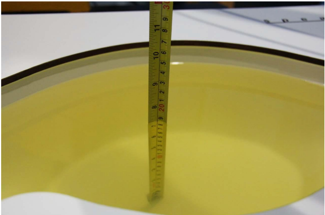
Picture 7-10: Liquid depth in the Flat Phantom(2450MHz)
