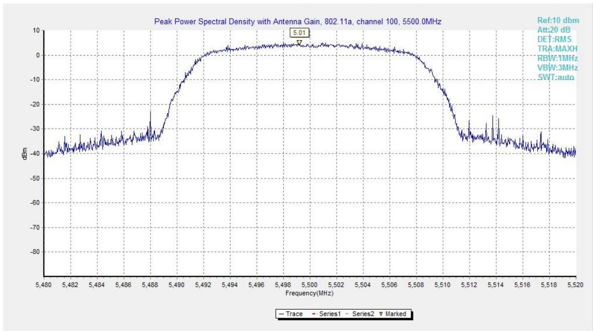
Fig. 7 Power Spectral Density (802.11a, 5500MHz)
