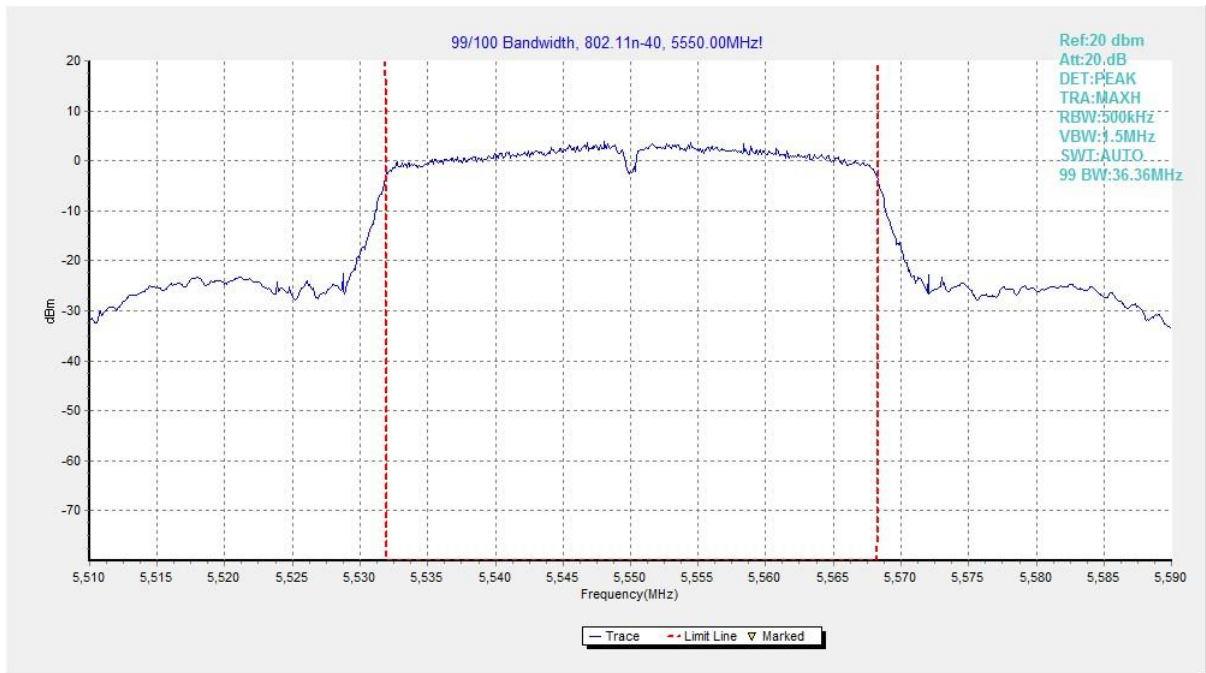
Fig. 50 99% Occupied Bandwidth (802.11n-HT40, 5550MHz)
