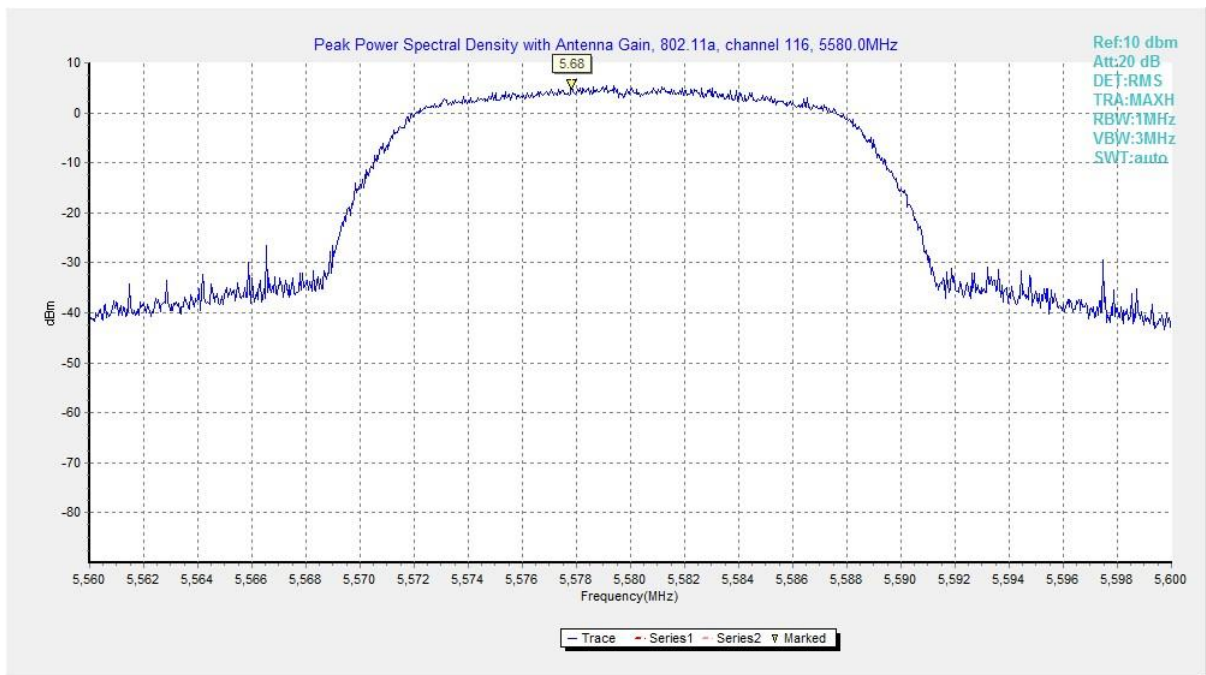
Fig. 8 Power Spectral Density (802.11a, 5580MHz)
