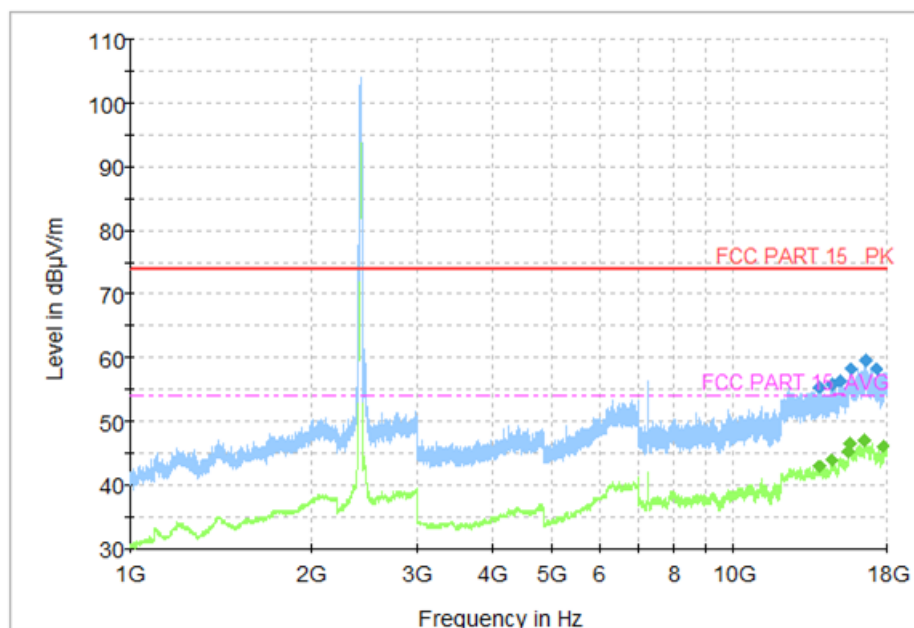
Fig.60 Radiated Spurious Emission (802.11n HT40, CH3, 1 GHz~18 GHz)
