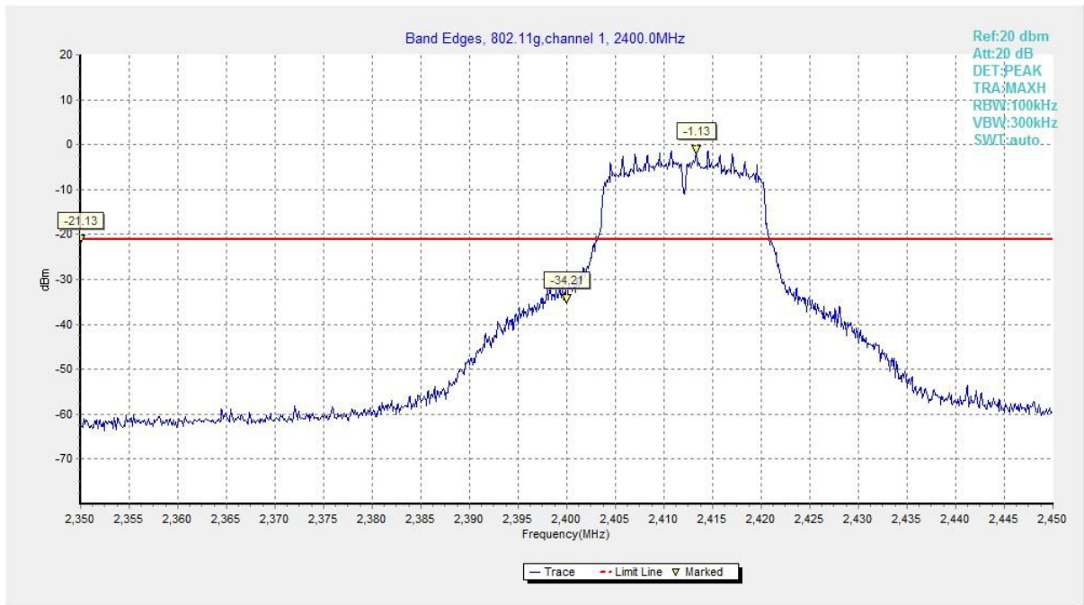
Fig.27 Band Edges (802.11g, CH 1)
