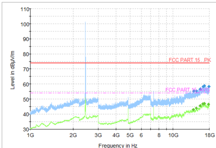
Fig.46 Radiated Spurious Emission (802.11b, CH6, 1 GHz-18GHz)
