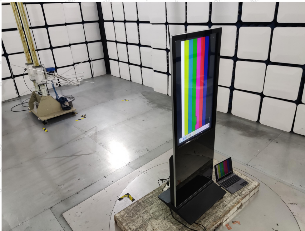
Photo of Radiation Emission Test
