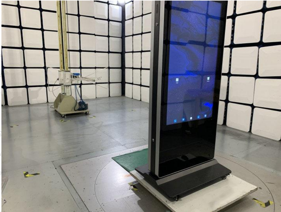
Photo of Radiation Emission Test
