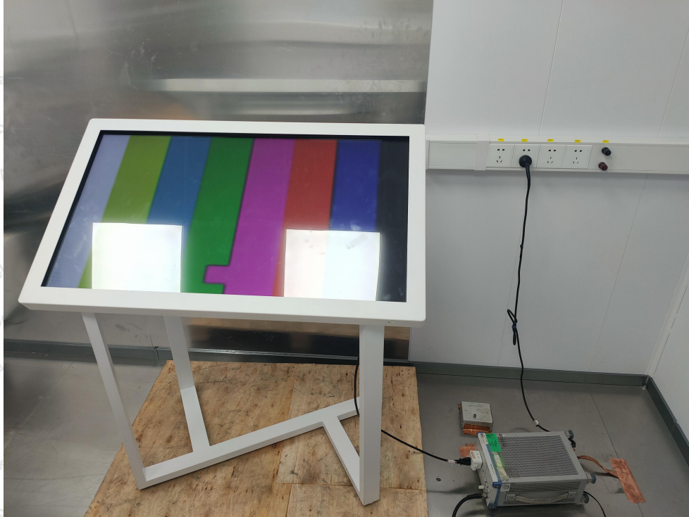
Photo of Radiation Emission Test (below 1GHz)
