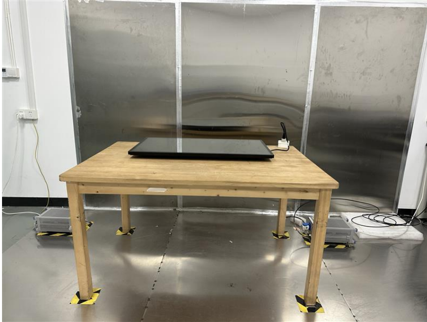
Conducted Emissions at AC Power Line (150kHz-30MHz)
