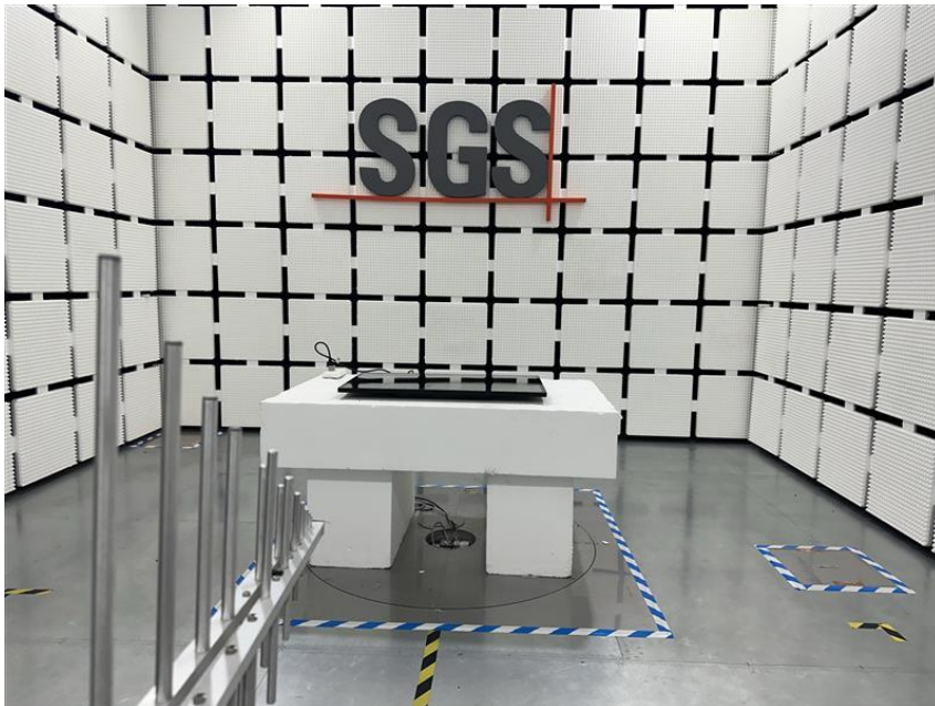
Radiated Spurious Emissions Below 1GHz
