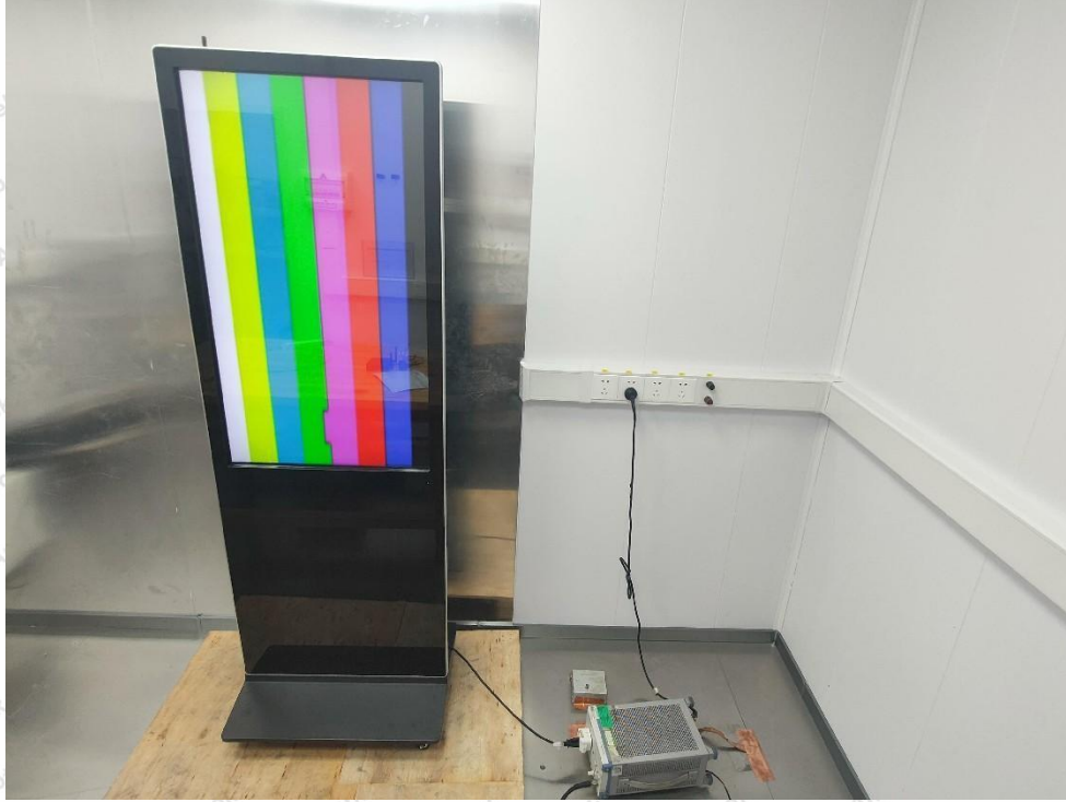
Photo of Radiation Emission Test (below 1GHz)
