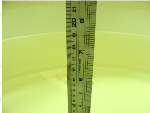
Photo of Liquid Height for Body SAR
