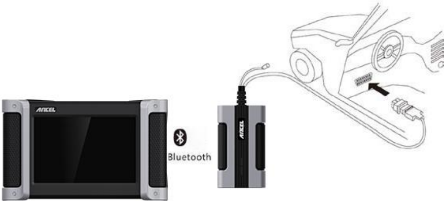
Figure 3.2-2 Connection of non-OBD-II port
