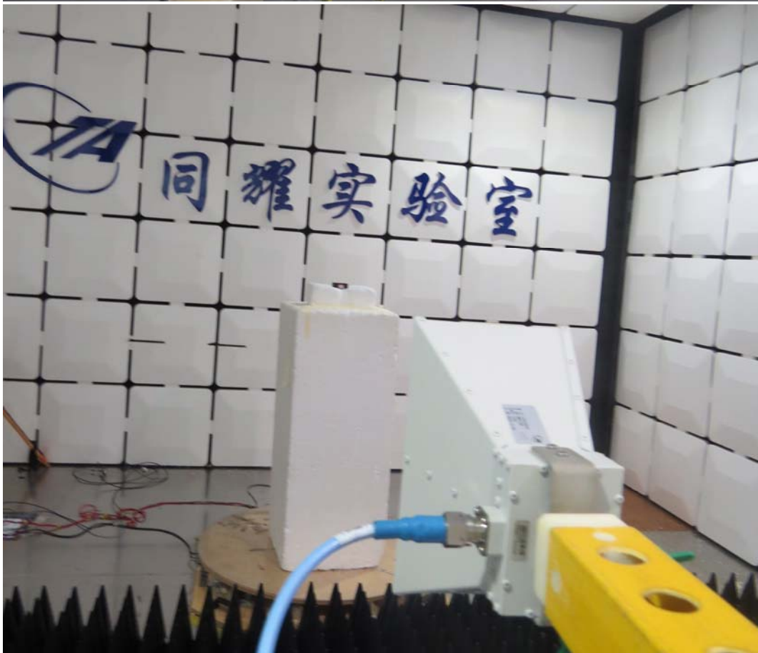
Picture 2 Radiated Spurious Emissions Test setup
