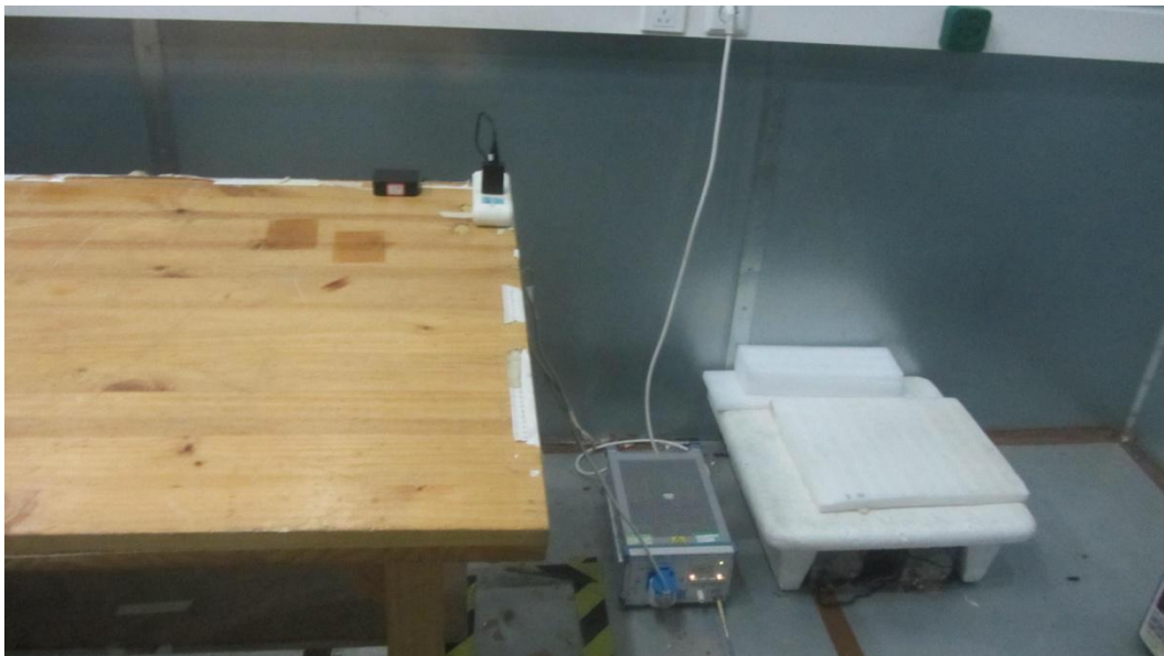
Picture 3 Conducted Emission Test Setup
