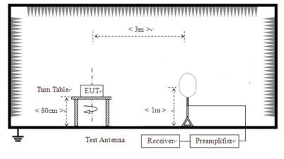
For radiated emissions from 30MHz to1GHz
