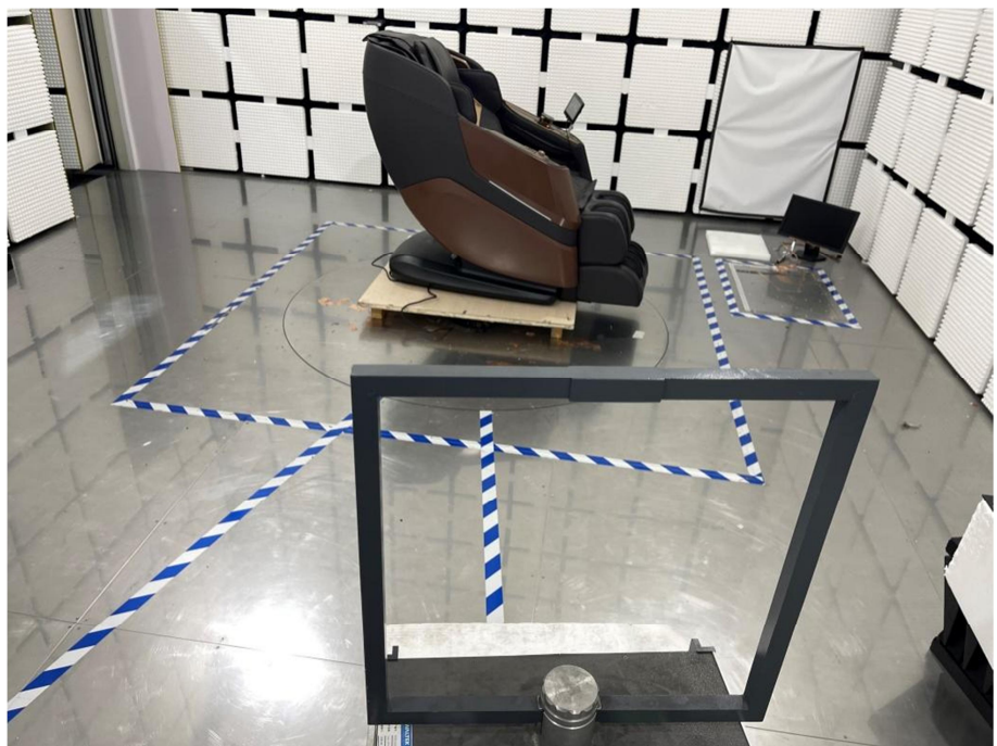
Radiation Emission Test Setup (Below 30MHz)
