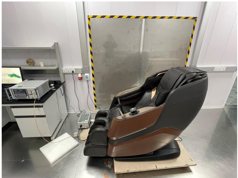
Conducted Emission Test Setup
