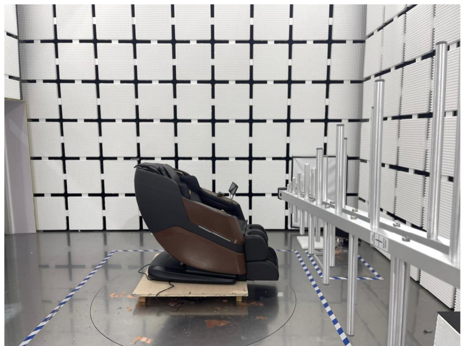
Radiation Emission Test Setup (30MHz to 1GHz)
