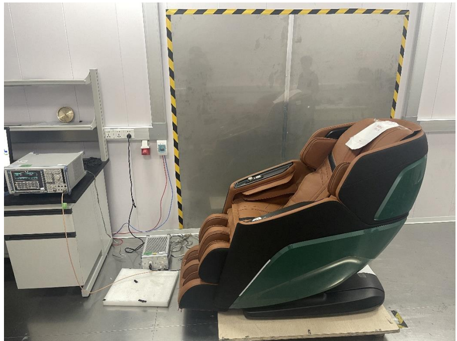
Conducted Emission Test Setup
