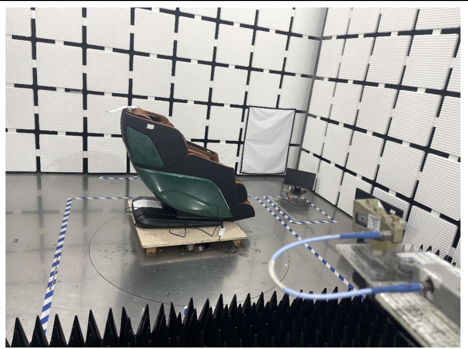
Radiation Emission Test Setup (Above 18GHz)
