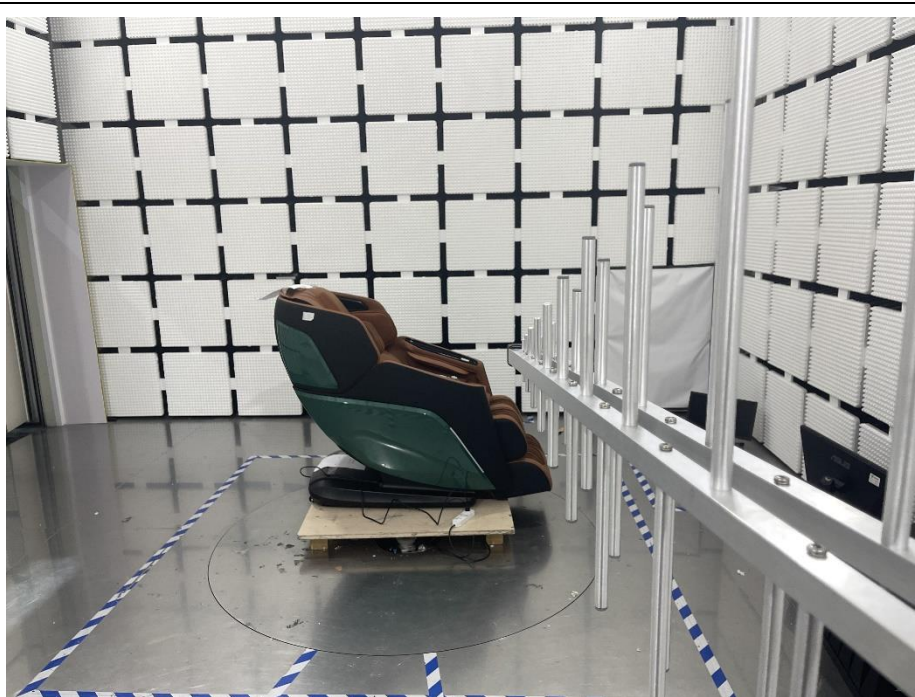
Radiation Emission Test Setup (30MHz to 1GHz)
