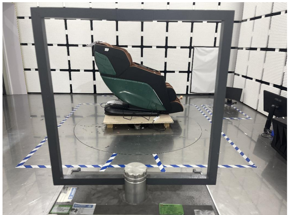
Radiation Emission Test Setup (Below 30MHz)
