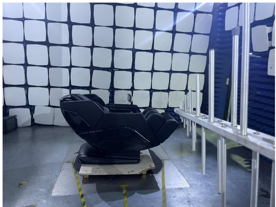
Radiation Emission Test Setup (30MHz to 1GHz)
