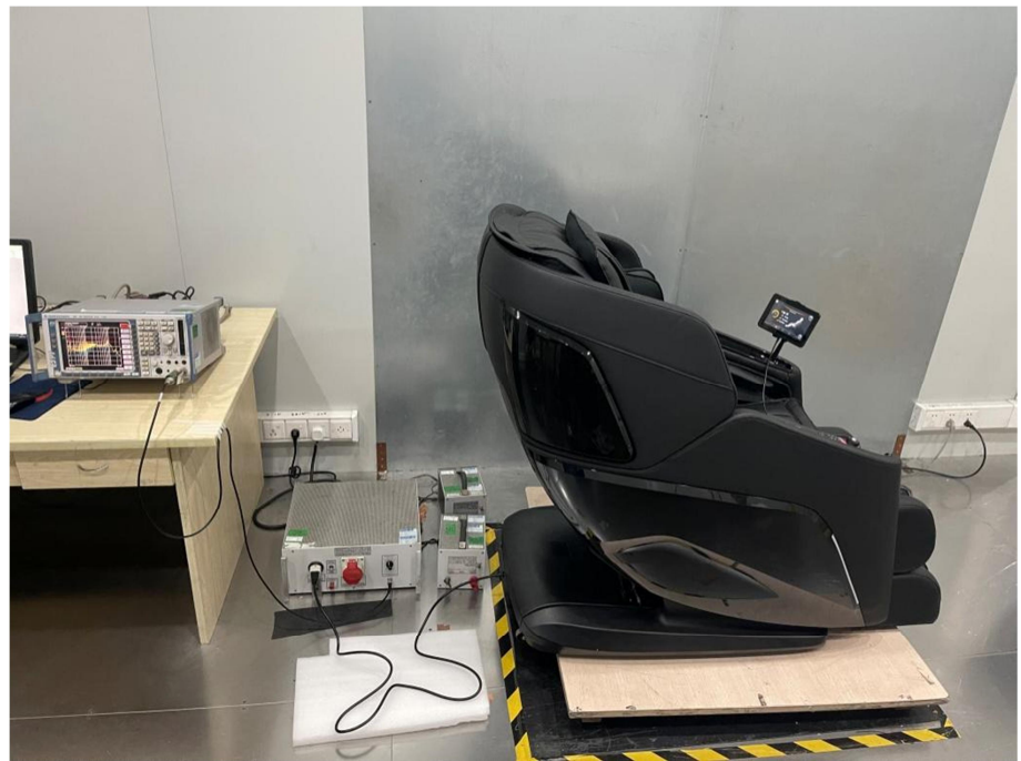
Conducted Emission Test Setup
