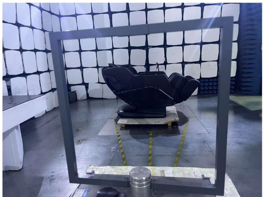
Radiation Emission Test Setup (Below 30MHz)
