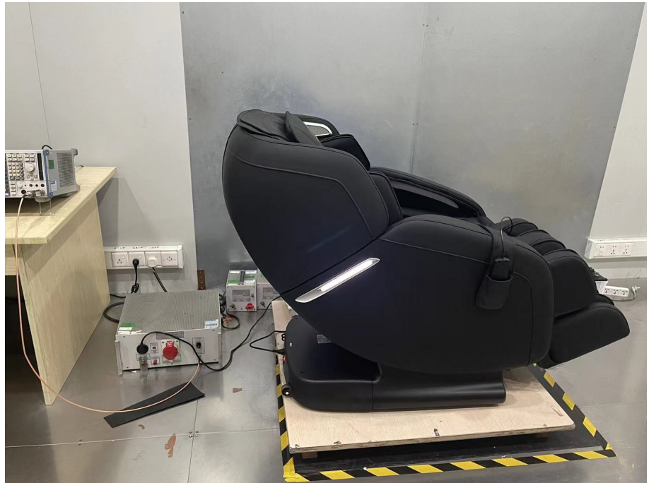
Conducted Emission Test Setup
