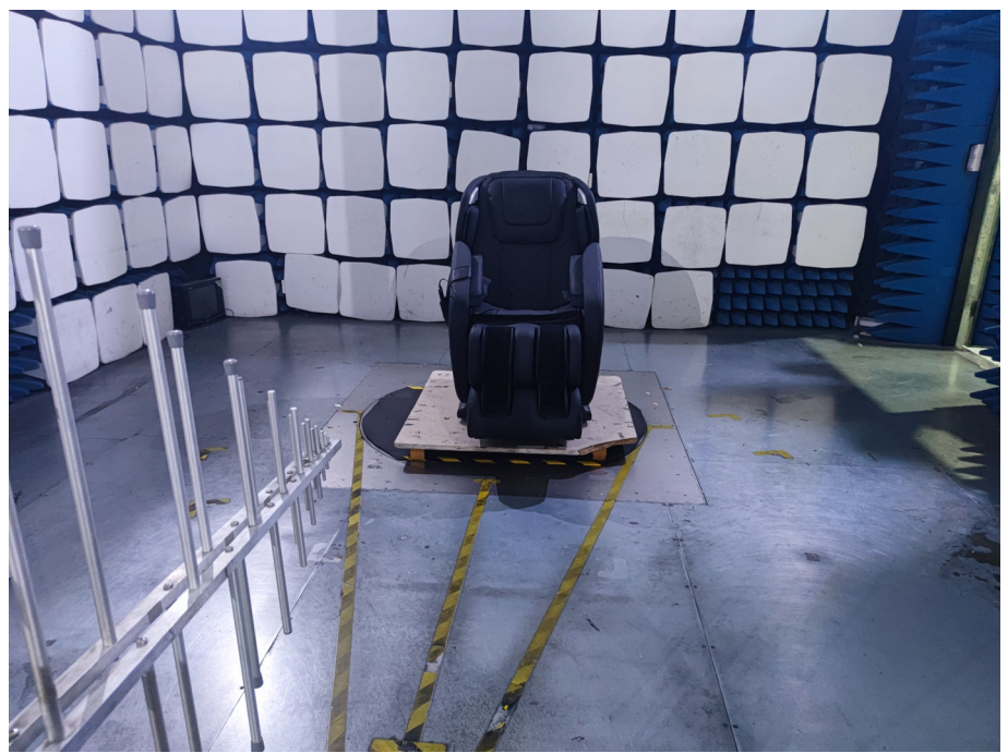
Radiation Emission Test Setup (30MHz to 1GHz)
