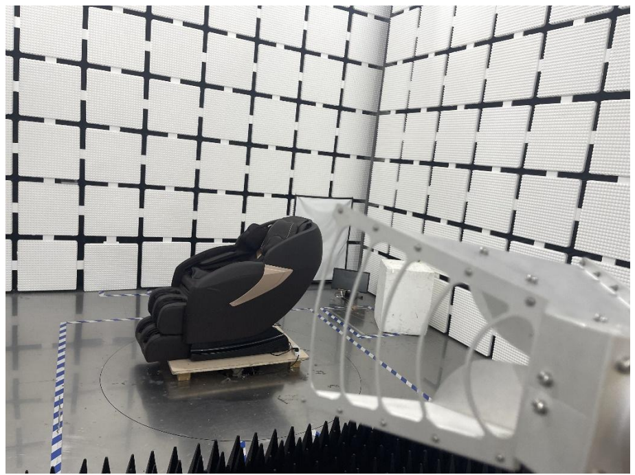
Radiation Emission Test Setup (1GHz to 18GHz)
