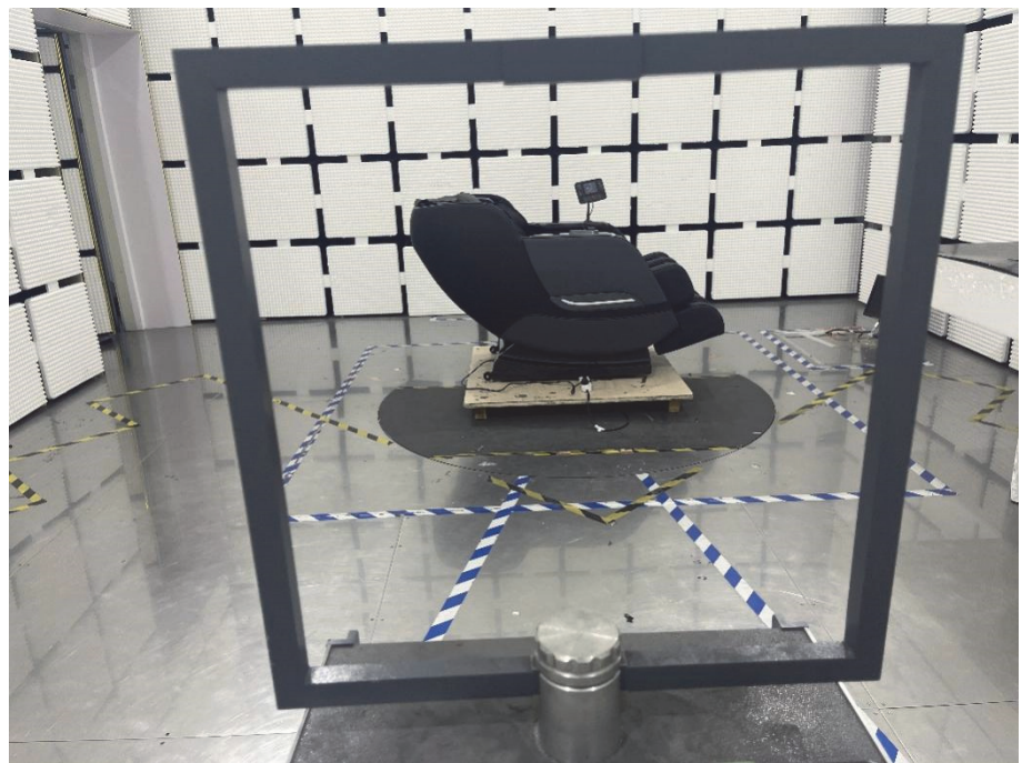
Radiation Emission Test Setup (Below 30MHz)
