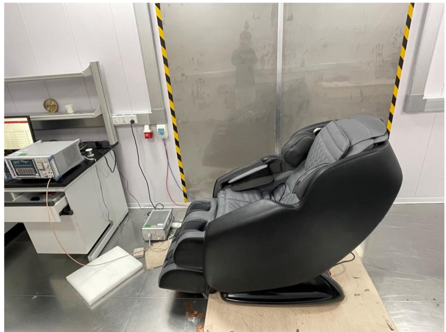
Conducted Emission Test Setup
