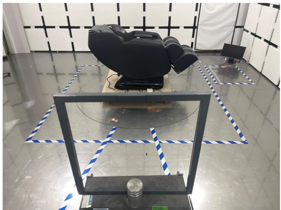
Radiation Emission Test Setup (Below 30MHz)
