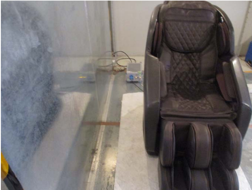
Conducted Emissions (Side View)
