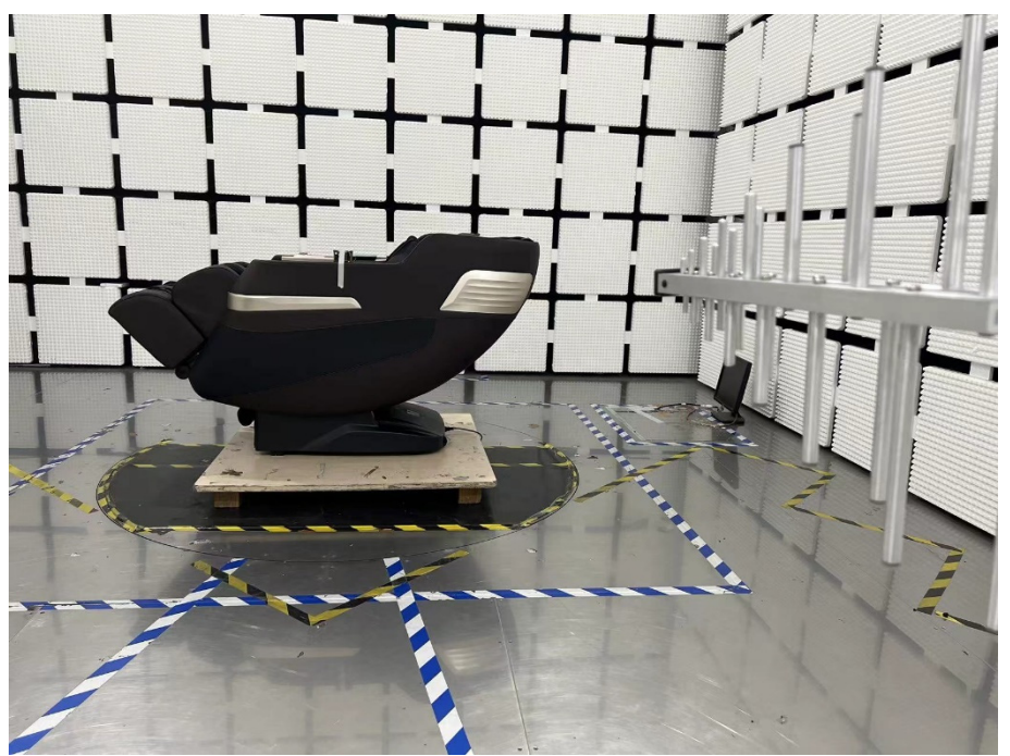
Radiation Emission Test Setup (30MHz to 1GHz)
