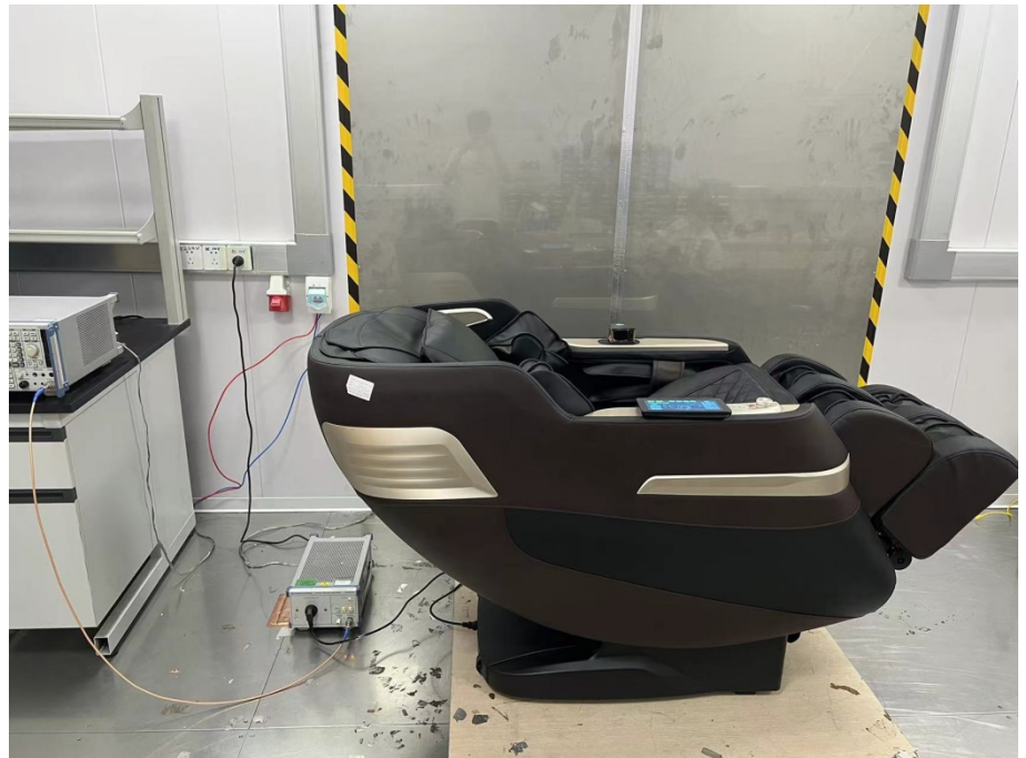
Conducted Emission Test Setup
