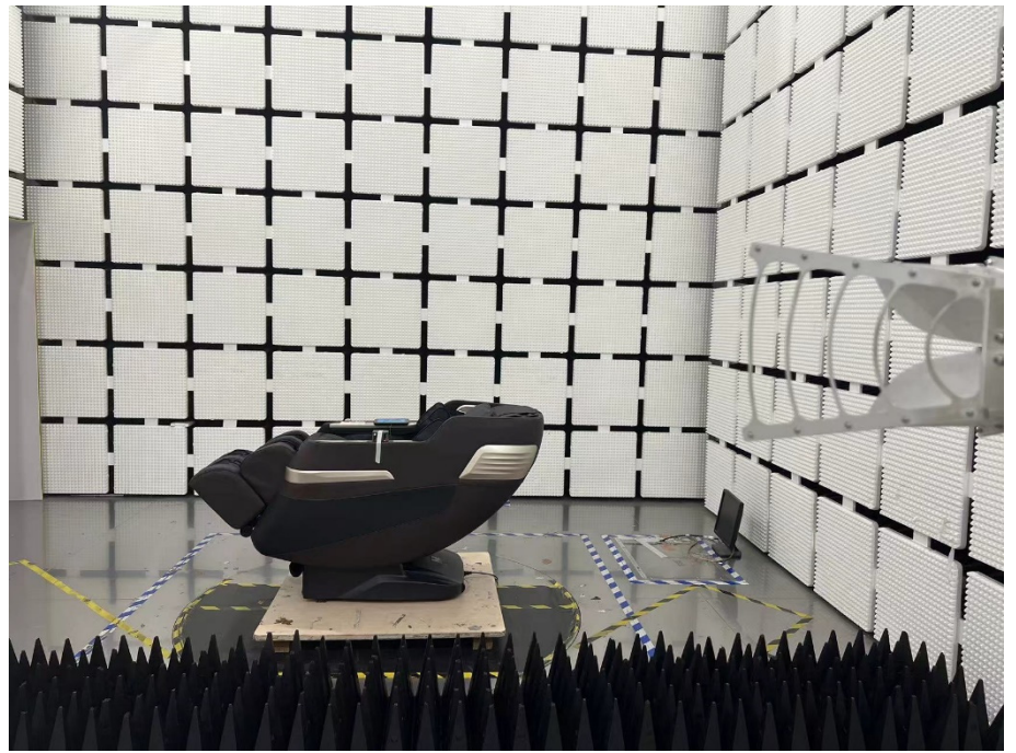
Radiation Emission Test Setup (1GHz to 18GHz)
