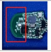
The antenna is PCB antenna.
