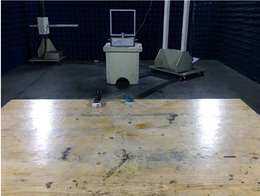
Photograph of set-up for Radiated Emission below 30MHz
