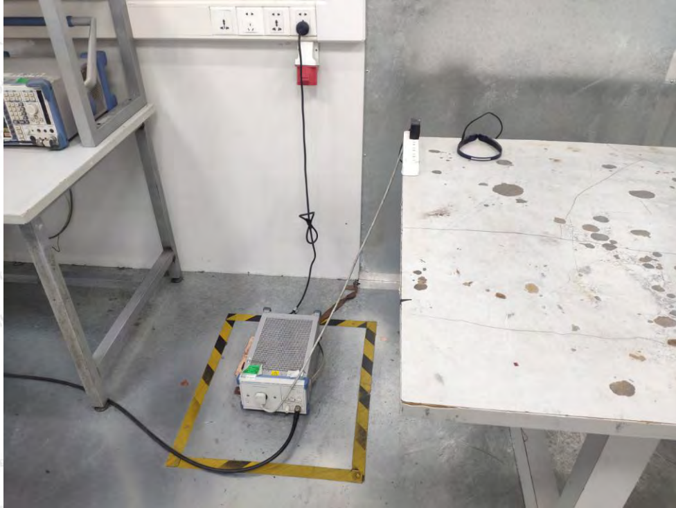
Photo of Conducted Emission Measurement
