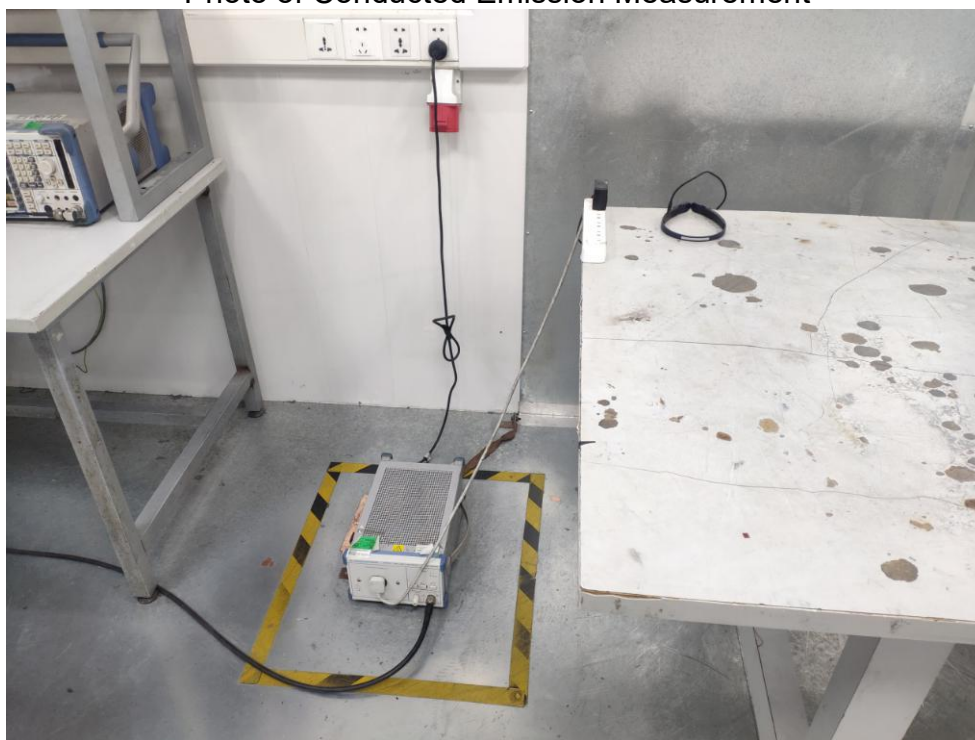
Photo of Radiation Emission Test
