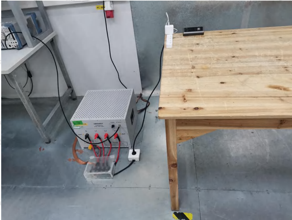
Photo of Conducted Emission Test
