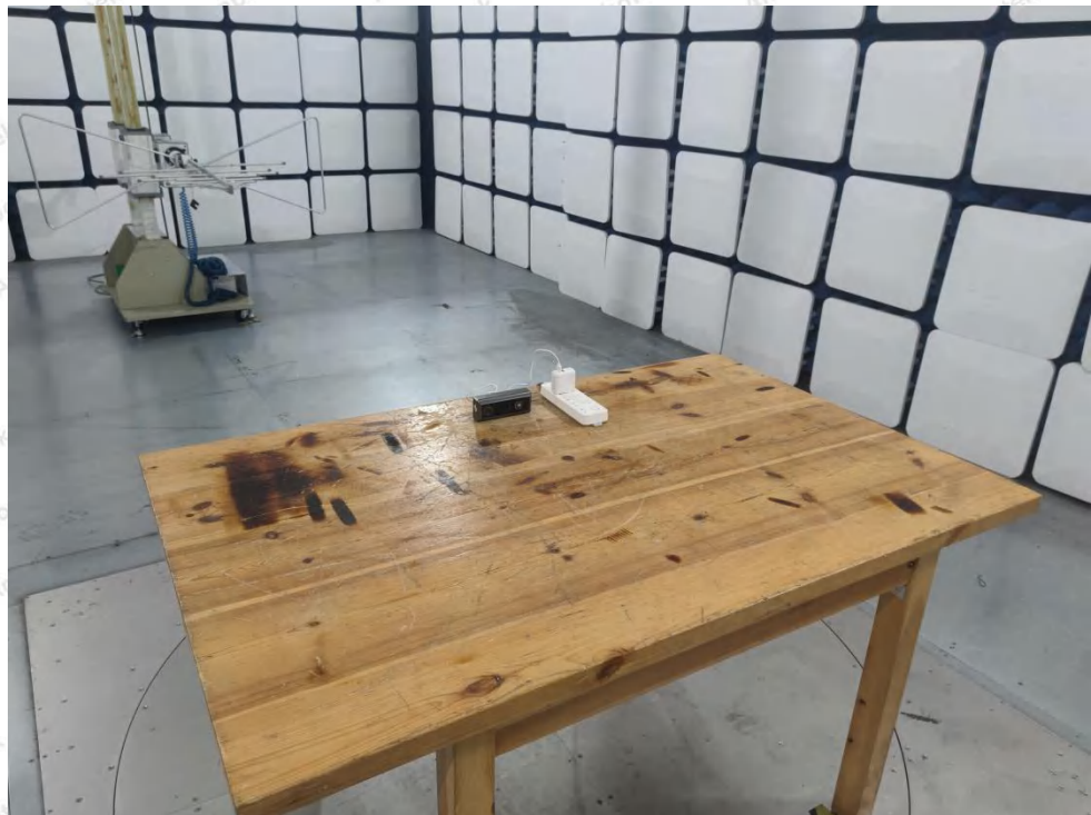
Photo of Radiation Emission Test
