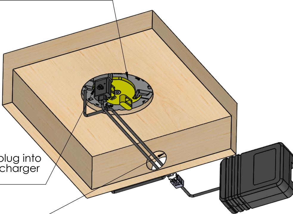
Connect USB plug into Wireless W-2 charger USB socket
