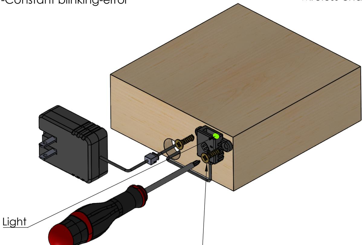
Screw in the USB HUB using a Philips screwdriver, using the screws provided
