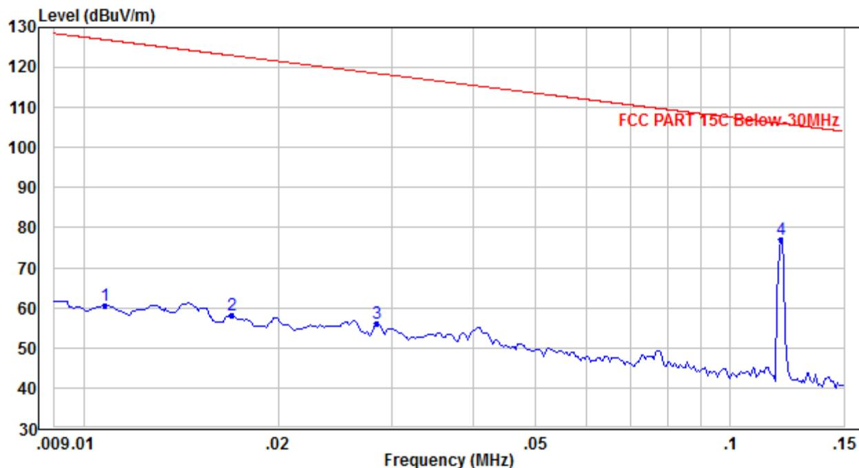
**Radiated Emission Test Data (150 KHz ~ 30 MHz):**
