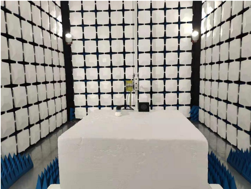
Above 1GHz for radiated emission test setup
