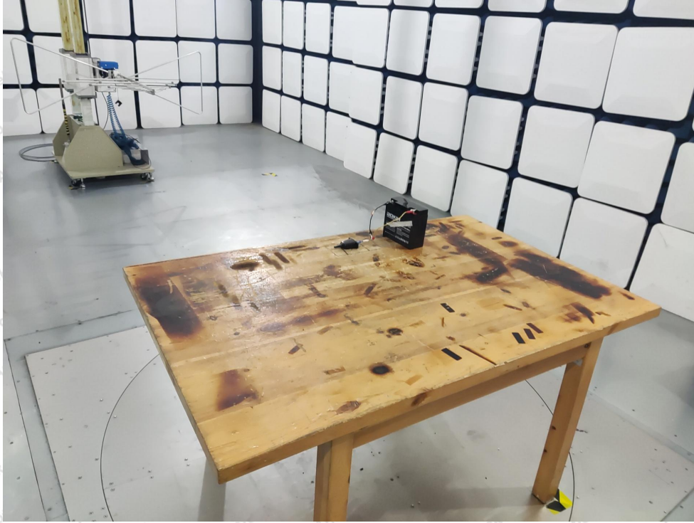
Photo of Radiation Emission Test (below 1GHz)
