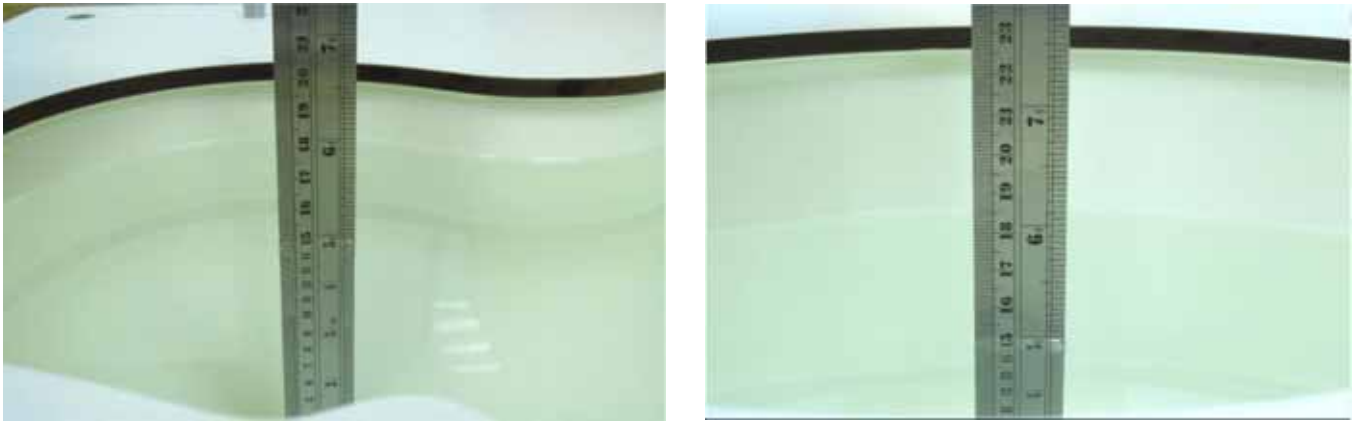
Figure D-1 Liquid Height for Head & Body Position (SAM Twin Phantom)
