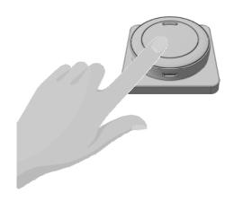
When the button is pressed, the indicator light flashes red and the device sends a message.
