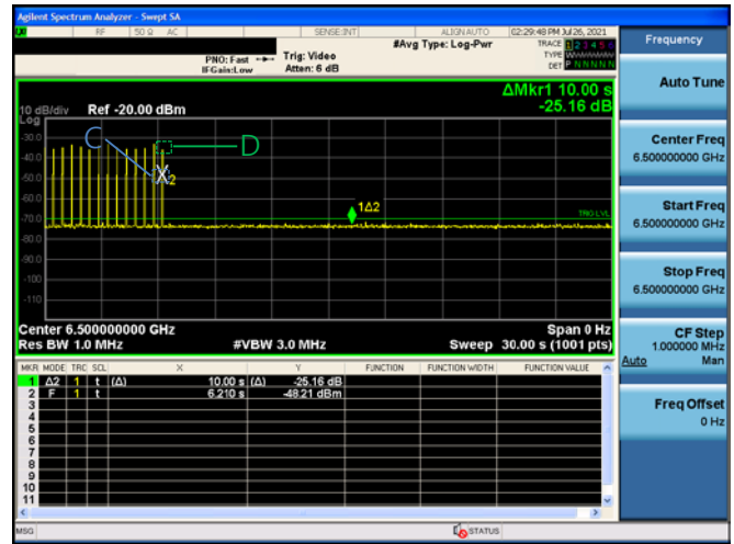
C: The receiver device ends the UWB link. D: The EUT cease transmission within 10 seconds.
