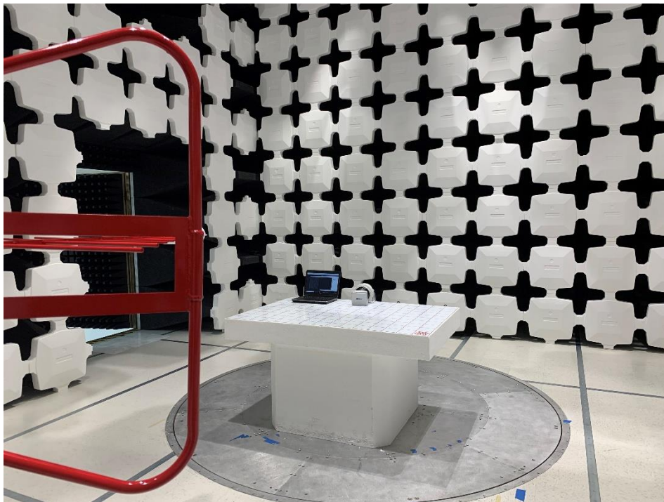
Radiated Emissions Below 1GHz setup – Front
