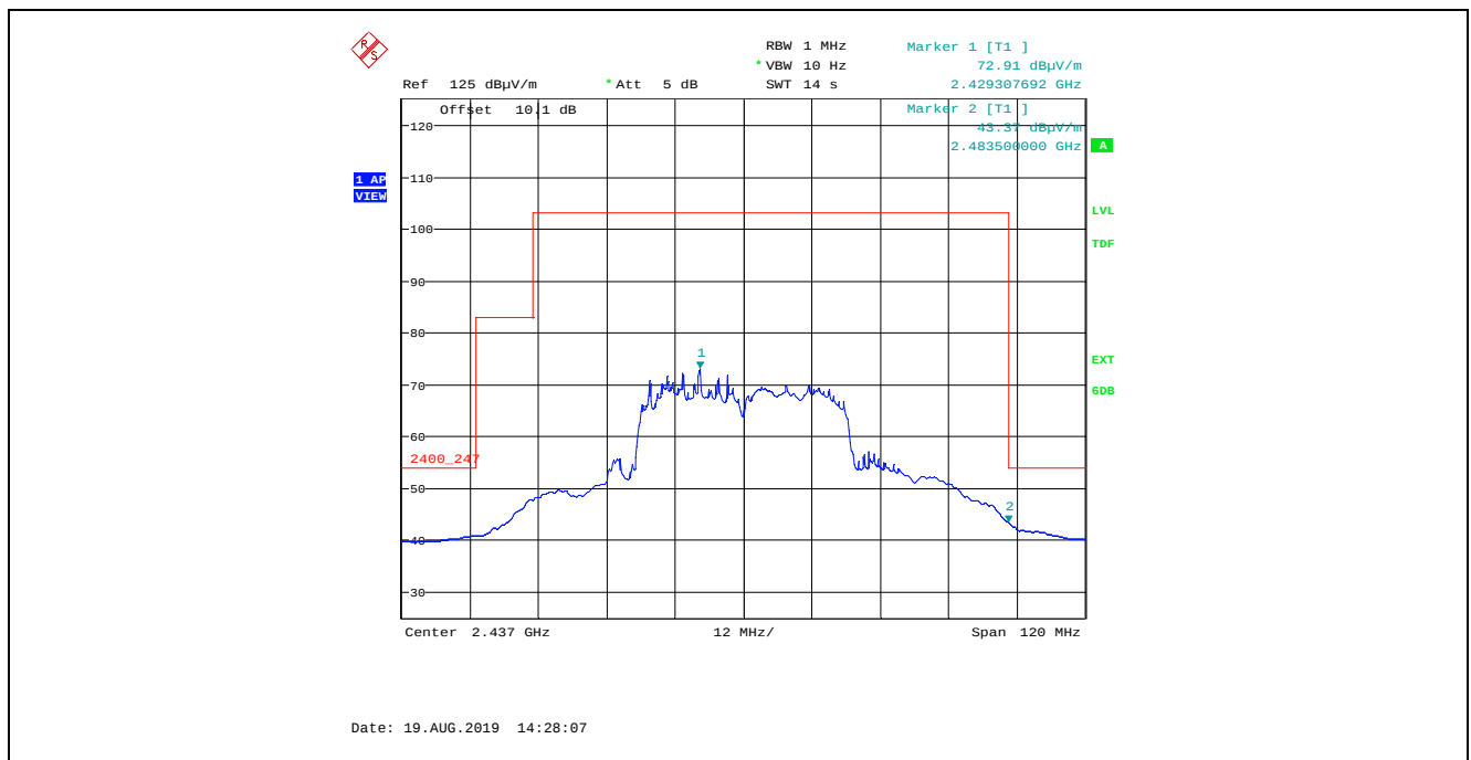
Plot 5.4.4.2.5.44. Band-Edge RF Radiated Emissions at 3 m, Horizontal Polarization, Average 802.11n HT40, 400 ns, MCS 7, 64-QAM 5/6 150.0Mbps, Power Setting 19, Channel 6, 2437 MHz
