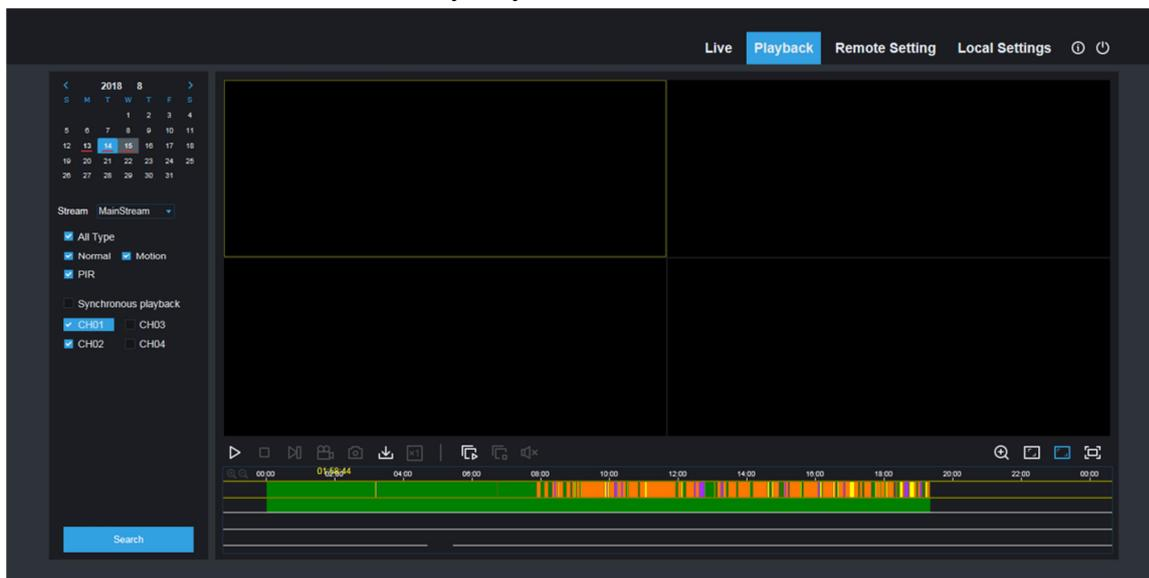
Click **Playback** to enter into Playback interface to remotely view the records in WIRELESS NVR HDD.
