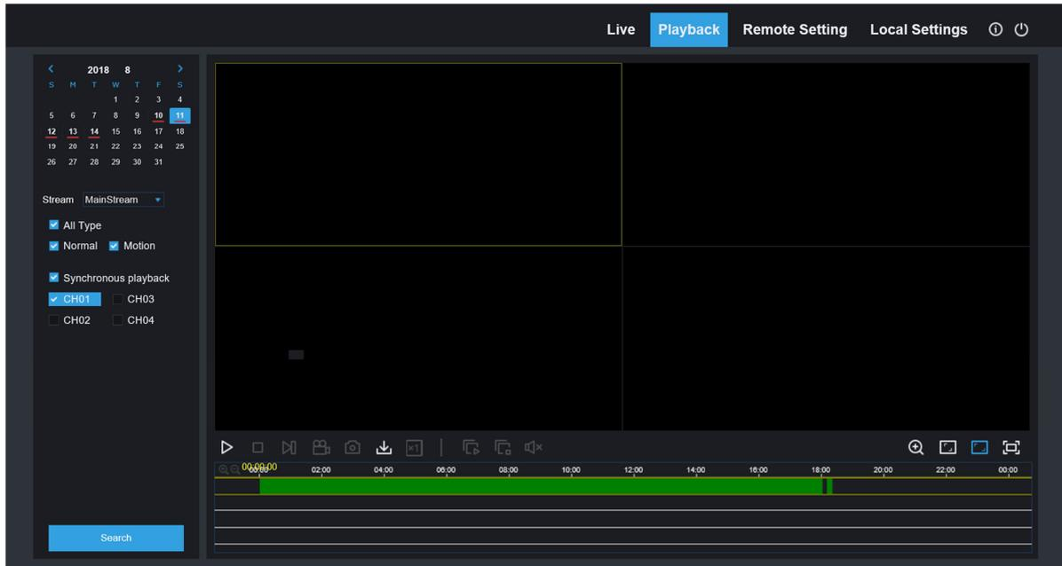
Before playback, choose to enable playback 4 channels synchronously. If you tick-select
