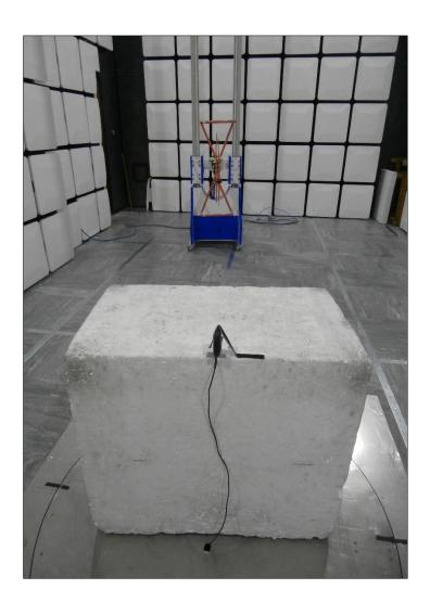
Figure 5 - Test Setup - 1 GHz to 13 GHz - Y Orientation
