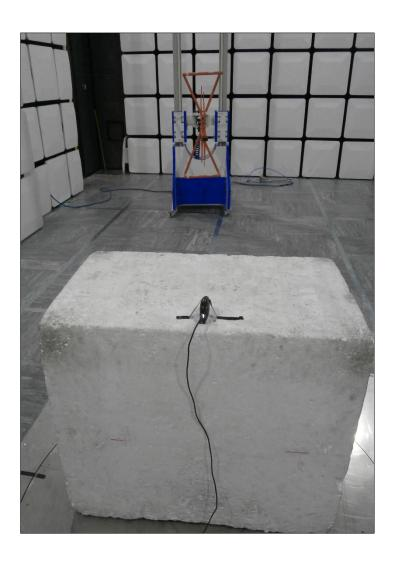
Figure 3 - Test Setup - 30 MHz to 1 GHz - Z Orientation
