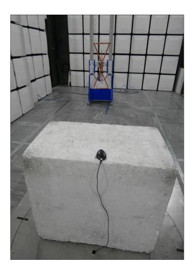
Figure 1 - Test Setup - 30 MHz to 1 GHz - X Orientation
