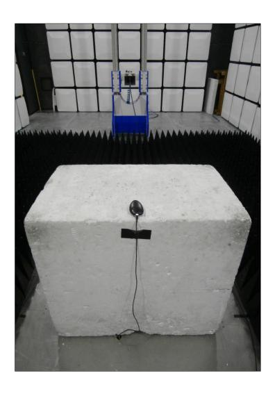
Figure 4 - Test Setup - 1 GHz to 13 GHz - X Orientation
