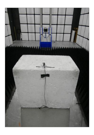
Figure 6 - Test Setup - 1 GHz to 13 GHz - Z Orientation
