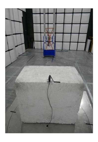
Figure 2 - Test Setup - 30 MHz to 1 GHz - Y Orientation
