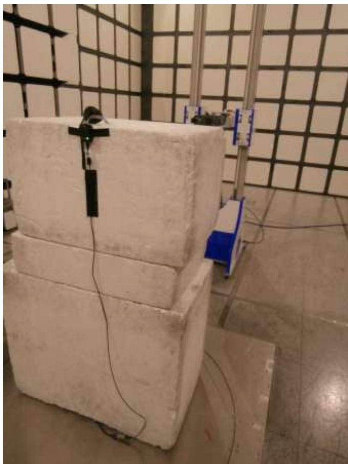
Figure 80 - Test Setup - 1 GHz to 25 GHz – Z Orientation
