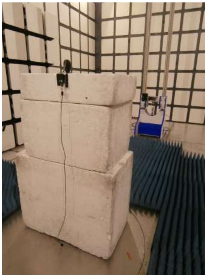
Figure 76 - Test Setup - 1 GHz to 18 GHz – Y Orientation
