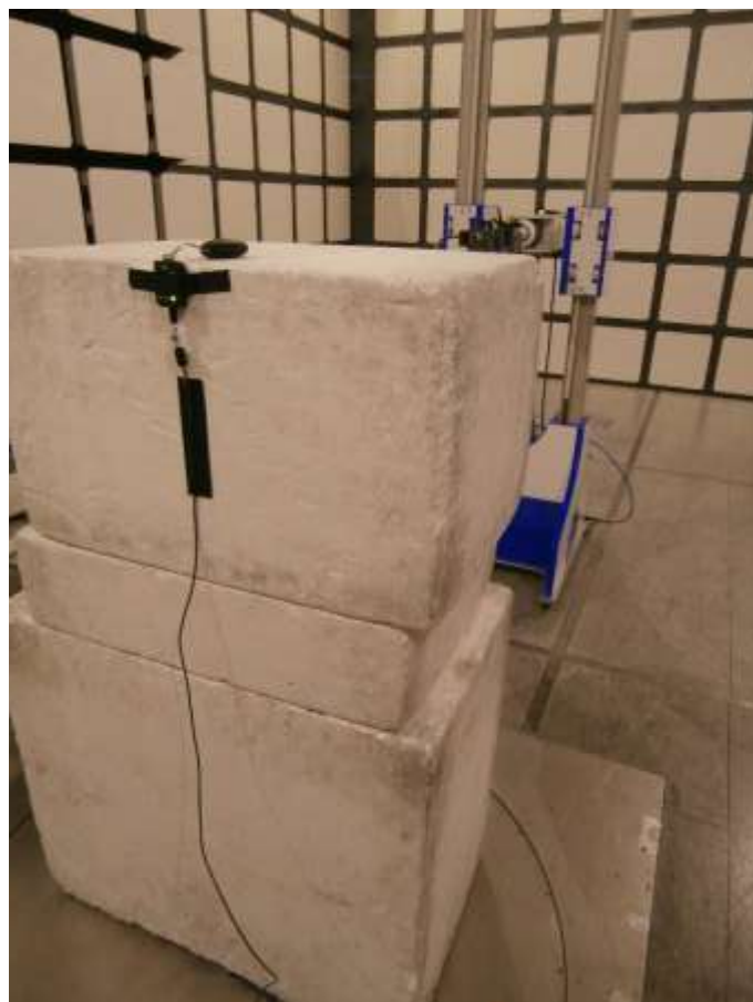
Figure 78 - Test Setup - 1 GHz to 25 GHz – X Orientation
