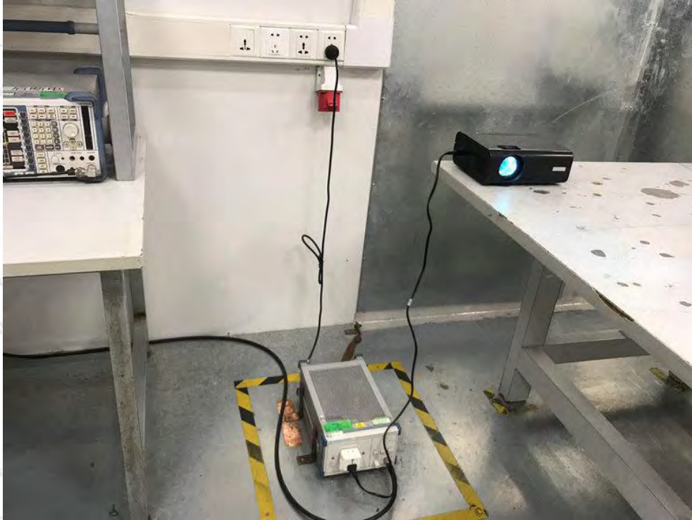
Photo of Power Line Conducted Emission Test
