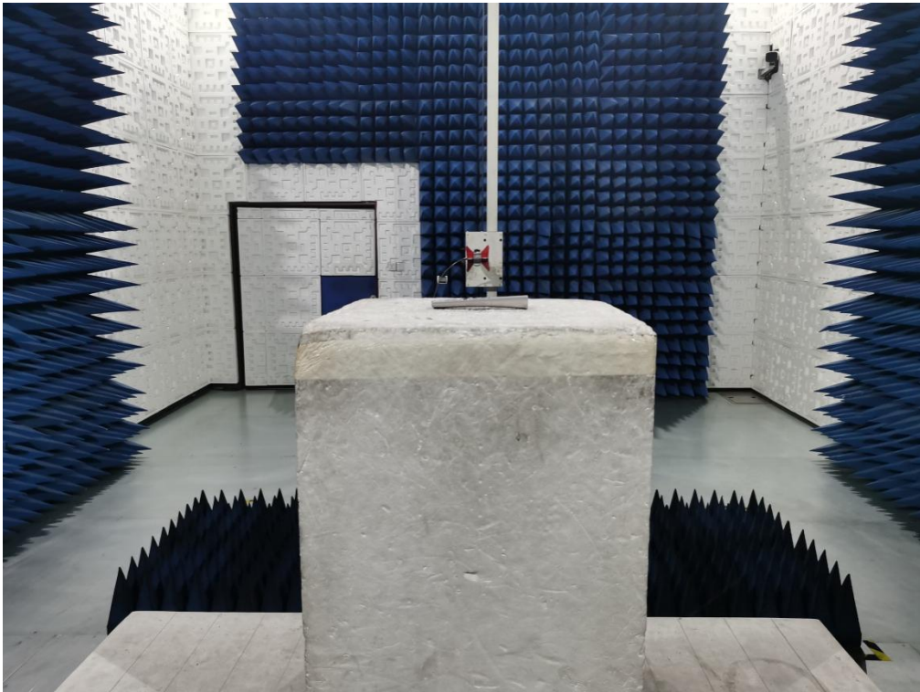
RADIATED EMISSION TEST SETUP ABOVE 1GHZ
